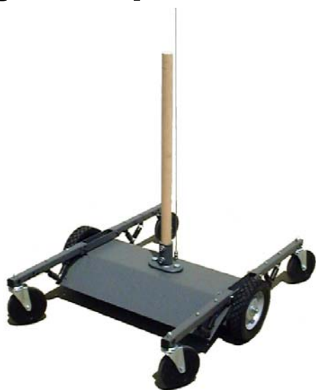
MAD ROBOT model MR2 5" casters front and rear, for flat, smooth surfaces to moderately rough terrain
