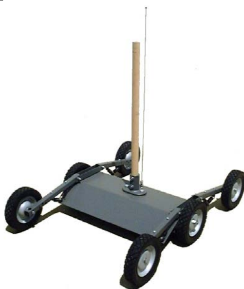
MAD ROBOT model MR3 8" x 1 \frac{3}{4} " Rubber tires, front and rear, Best for rough terrain, outdoors in dirt, packed gravel, grass or similar.
