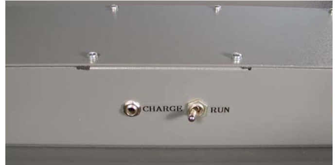
Close up of MAD ROBOT "Control Panel" showing the battery charging port and power switch.
