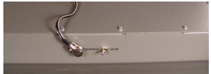
Charger connected to charging port. (The MAD ROBOT is normally NOT turned upside down to make this connection.)
