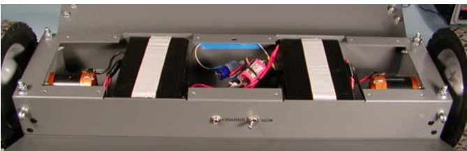
Maintenance panel removed to show interior of MAD ROBOT. Note the two motor/gearcase assemblies and the two 12V Gel-Cell batteries. The R/C radio receiver and the motor control circuitry are located in the center section.
