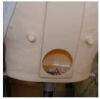
This target must be modified by cutting a 4" diameter hole in the rear of the target to access the interior. Then drill two  $\frac{1}{2}$ " diameter holes in the bottom of the target to match the holes in the flange fitting. Fasten the flange fitting to the target with the supplied screws, washers and nuts. The backing plate is not required for this target.
