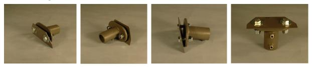
The SLP adapter is used with a variety of targets, as shown below. This adapter consists of an oval flange fitting and a metal backing plate as well as fastening hardware: 2 each of a  $\frac{1}{2}$ -13 x 1 $\frac{1}{2}$  Hex Cap Screw, a  $\frac{1}{2}$ ID x 1 $\frac{1}{2}$ OD Fender Washer and a  $\frac{1}{2}$ -13 Locknut. A  $\frac{1}{4}$ " Hex L-Key for the set screws is also included.
